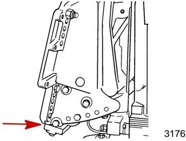
The anode requires periodic inspection, especially in salt water which will accelerate the erosion. To maintain this corrosion protection, always replace the anode before it is completely eroded. Never paint or apply a protective coating on the anode as this will reduce effectiveness of the anode.
