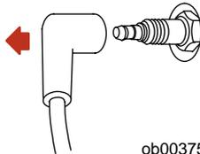
2. Remove the spark plugs to inspect. Replace spark plug if electrode is worn or the insulator is rough, cracked, broken, blistered or fouled.
